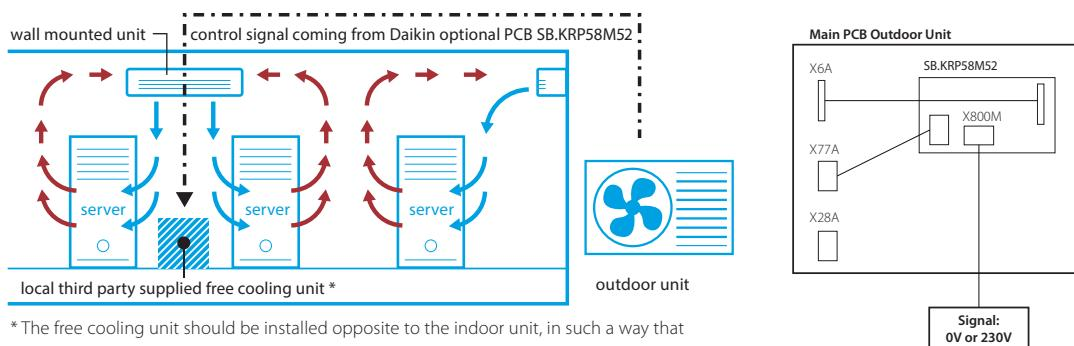
With the free cooling 230 V signal supplied through optional control board SB.KRP58M52 **available**
