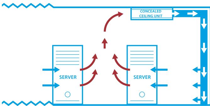
Use concealed ceiling units to distribute cold air where needed (down and to the suction side of the servers).
